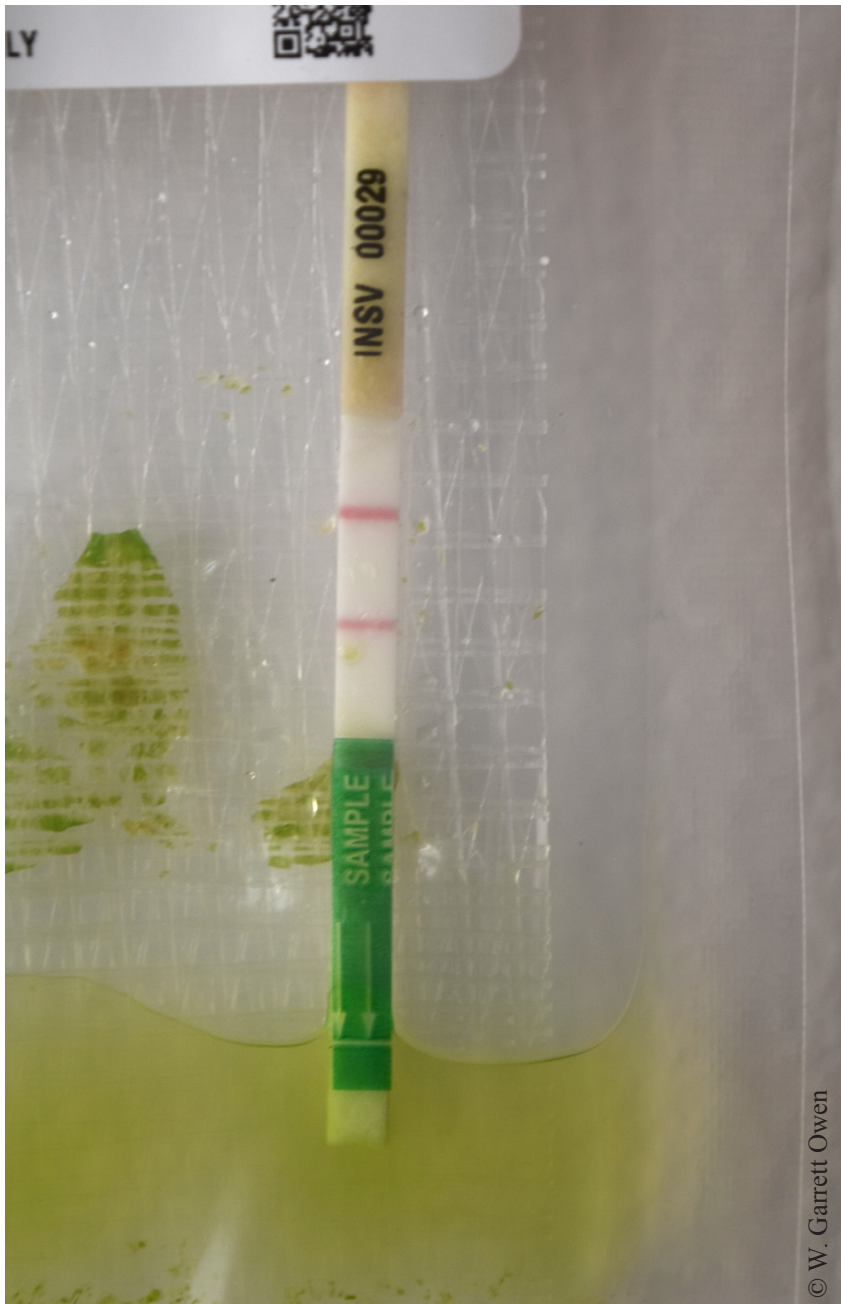
Figure 4. A confirmed INSV infestation with an enzyme-linked immunosorbent assay (ELISA) test. Note the double lines.
