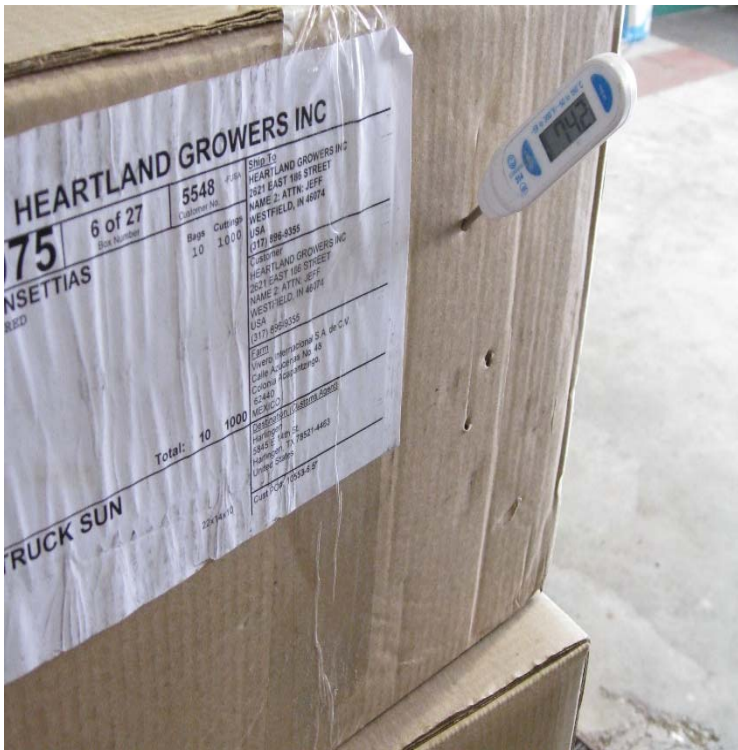
Figure 6. The temperature of a box containing cuttings is being measured.
